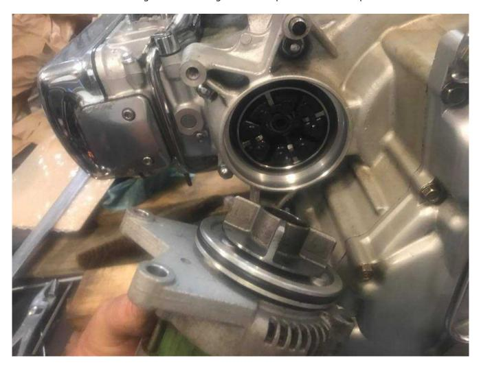
Put a little oil on the o-ring before pushing it into the case
