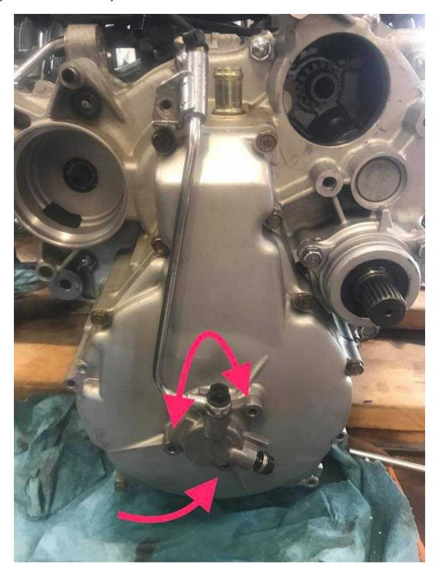
Tighten the bleeder tube holder bolt
