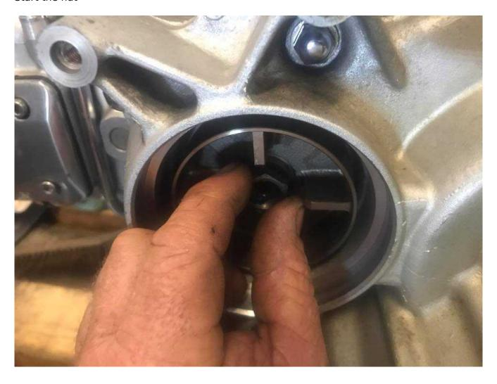
Yep, back to the u joint, pry bar holder down method again to keep the alternator gear from turning so I could torque it
