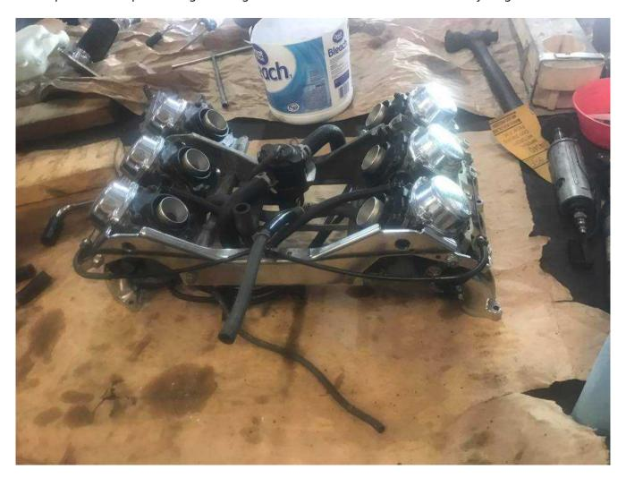
And eliminate a bunch of vacuum lines, and other unnecessary parts. Drive some 14 mm freeze plugs in to plug the holes and add the chrome back over them
