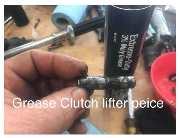
Place it in the center of the Clutch lifter plate and tighten the bolts evenly so it moves freely, if not start over until it moves freely
