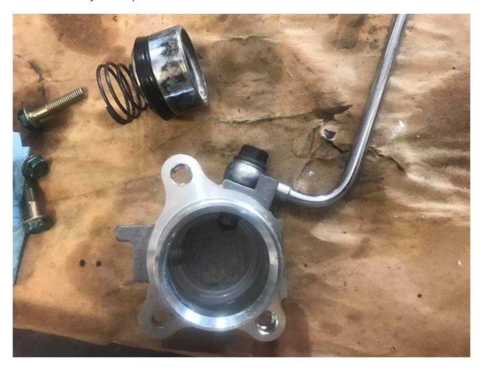
Poured a little brake fluid in it and rubbed it around the edges to Lube it for the piston
