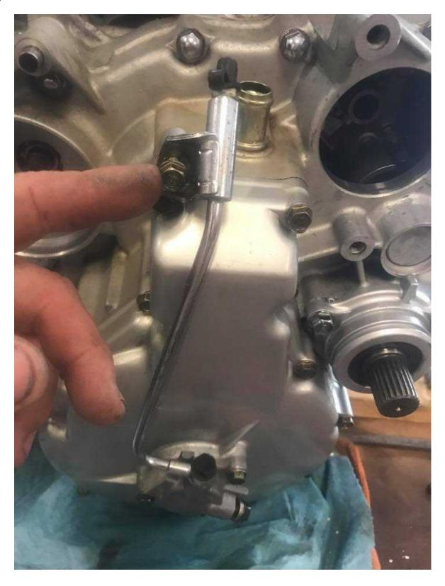
Install the alternator drive housing
