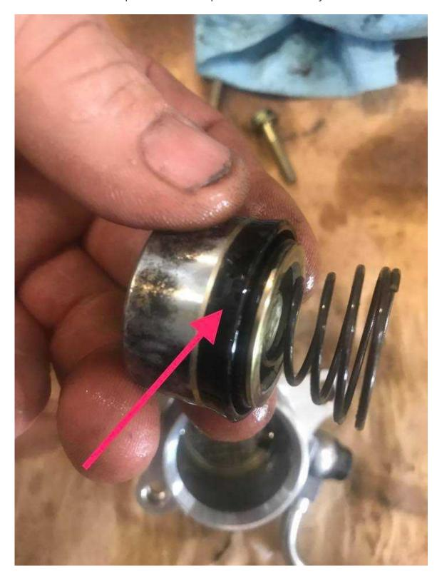
Once the piston is back in add a little grease into the Clutch rod hole
