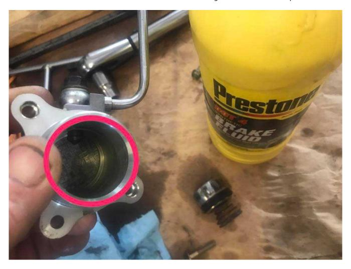
Put some brake fluid on the piston seal to help it slide back in easily
