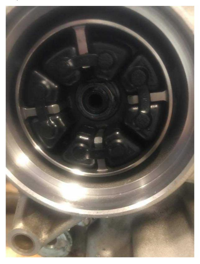
Install the alternator making sure the fins go into the spaces of the dampers
