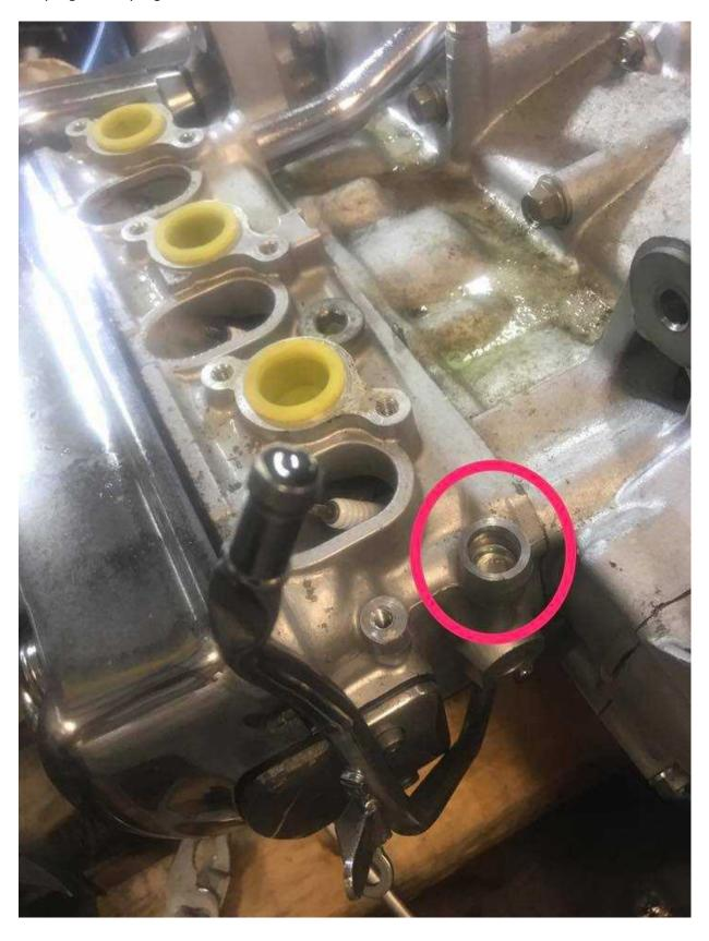
Squeeze some tubes and fill em with JB Weld to plug em off
