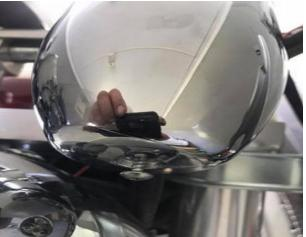
(left) After you push the new bulbs into the rubber holders turn the key on and make sure they work. They only work when put in one way, as you can see above I have one in right and one in wrong. No way to tell till you try em. So don't put it all back together before you try em.
