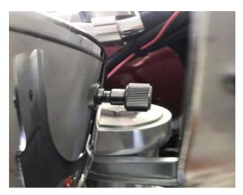
Install the trip meter knob making sure you align the flat spots.
