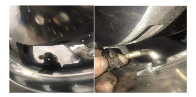
(left) This is a OEM stem, the metal part of the stem stops right where it meets the rim. They put a little plastic crutch under it to keep it from breaking off B.
