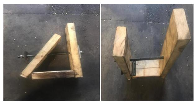
(Left) The hinge lets it fold on the short side to push the bead over on the rim.
