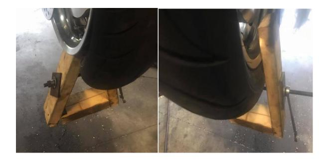
$({\rm left})$  I have 2 nuts together so this side I can turn with my impact wrench without the nut moving and making my socket too short
