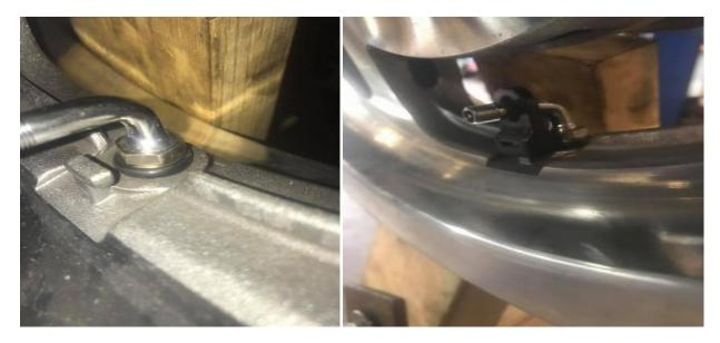
(left) Just enough to squash the rubber washer a little, there is also a rubber washer on the bottom inside the rim so it will seal without over tightening it and splitting the rubber washer.
