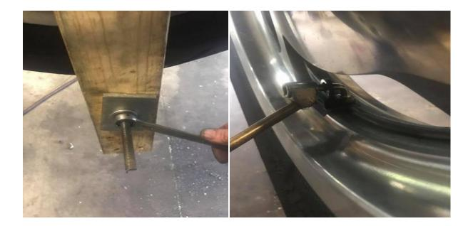
(left) Then loosen the nut on the back and remove the Mo Sheen
