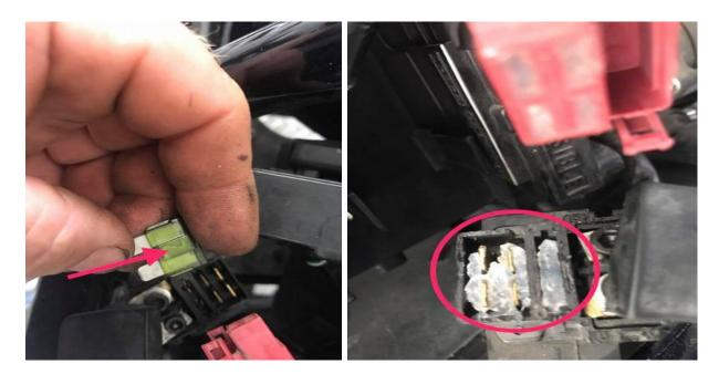
(left) This is the 30 amp fuse for the starter relay, when the fuse is blown the small metal strip shown by the arrow will be severed disconnecting the connection and will have to be replaced. If it ever blows and your bike won't start and you don't have a replacement, you can turn the key on and cross the 2 terminals under the Allen screws with a screwdriver to get the bike started to get you home.
