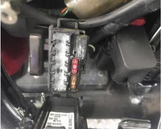
(left) I use my pocket knife to scrape the corrosion of the fuse blades so they make the best connection possible
