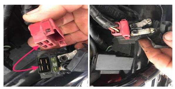
(left) This connection is the top of the starter relay. Clean the terminals on both sides with some electronic cleaner to remove any corrosion.
