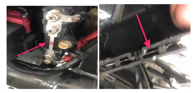
(left) This is the main fuse. It is a 50amp blade fuse, removed it and cleaned the contact areas then replaced it and put a dab of dielectric grease on the top to keep the moisture off it.
