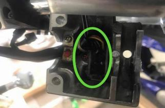
(left) Time to put it back together, make sure your button is hitting the contacts when out and heading towards the others when pushed. Once you snap the pieces back together I put a little dielectric grease around the white part of the button end so when I drop it back in the hole it will seal the end from moisture coming in around the button
