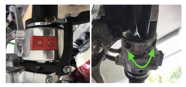
(left) Gonna pull this off and clean and waterproof these switches. 1st step: disconnect the Battery
