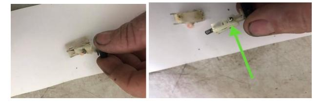
(left) Hold the bottom and lift the button out. Do this on an area that if the little ball comes out you can find it. Doesn't always pop out but when it does, the hunt is on.
