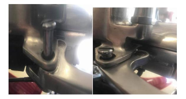
(left) Insert the pivot bolt in the hole. If the threads don't want to line up squeeze the Clutch handle a couple times to push the plunger into the master cylinder so it will seat.
