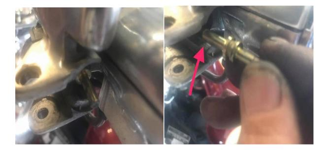
(left) Need to remove the plunger rod that goes into the master cylinder.
