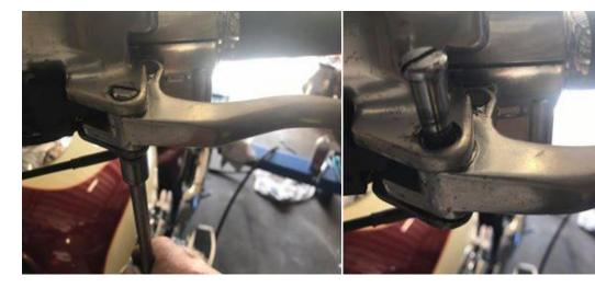
(left) Remove the 10mm nut off the pivot bolt
