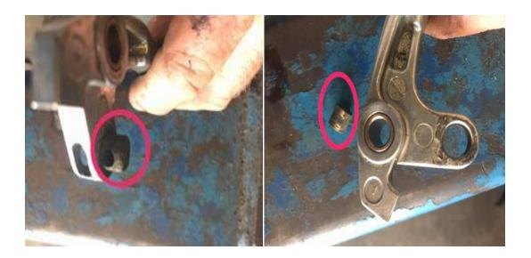
(left) More corrosion, need to pop the bushing out and clean it up (right) Lots of corrosion and grinding around it.
