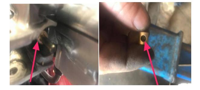
(left) Push the plunger rod back into the master cylinder making sure it goes into the rubber boot. Twist it to make sure the boot doesn't bind
