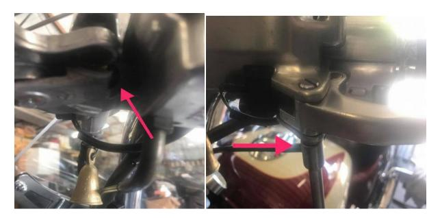
(left) Check to make sure the rubber boot isn't binding.
