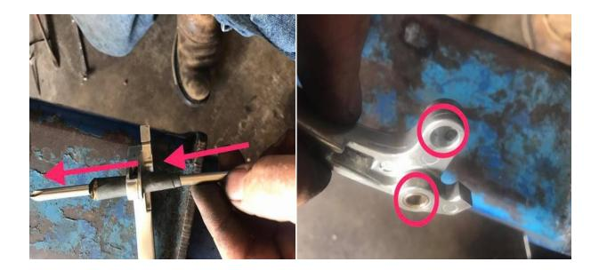
(left) Slide it all the way thru so it looks like this. Spin the handle around on the sandpaper so it will clean the corrosion and dirt off the inside of the hole.
