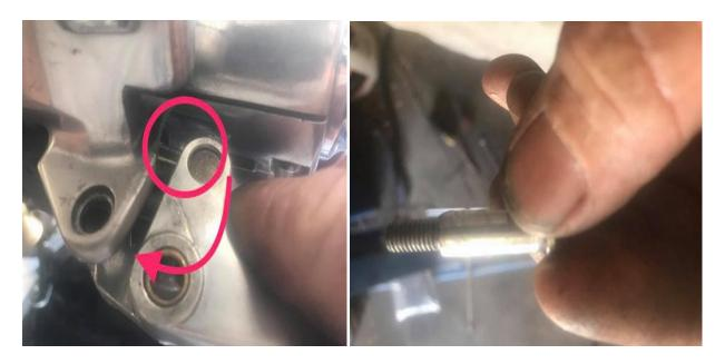
(left) Once the rod is into the bushing pivot the handle around so the pivot bolt hole lines up (right) Lube the outside of the pivot bolt.
