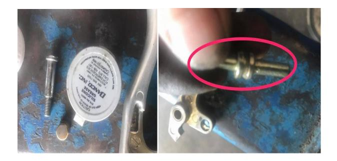
(left) I'm using a silicone grease to lube the pivot parts and bushings.
