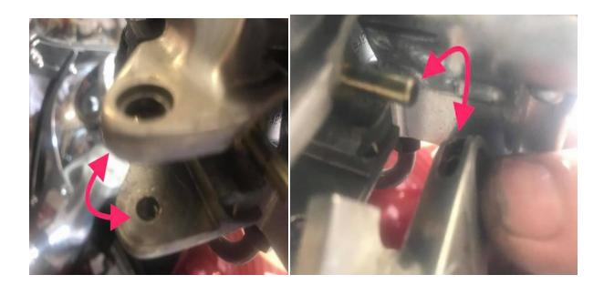
(left)Put a little lube on these parts that the handle slides on.
