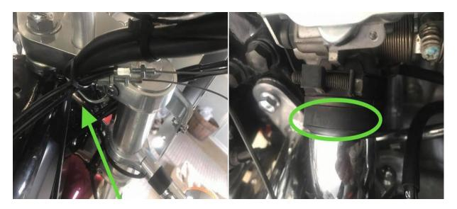
(left) I zip tie the throttle cables up out of the way so nothing hangs up on them and damages them (right) Didn't get a good picture here but there are 8mm clamps on the intake runners. Loosen all the lower ones.
