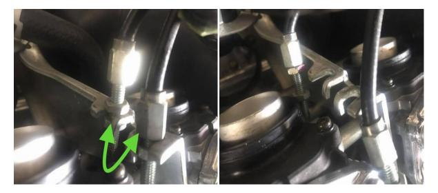
(left) Loosen the adjusters so you can get the cables out of the holders to make slack to release the throttle cables. You can mark the settings with paint or a marker if your unsure on how to adjust them when putting back together.
