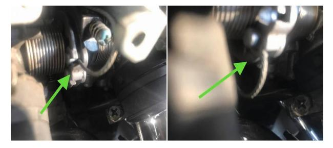
(left) Pivot the cable to the slot and it will slide out
