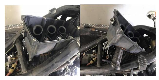
(left) Start lifting the back of the box out while making sure the tubes are coming free from the carbs. Don't worry if the clamps come off you can get them once the box is out of the way.
