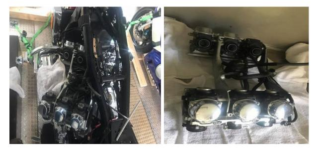
(left) Start working the carb assembly out the left side. Go easy and watch for hoses and wires that may try to get tangled in them.
