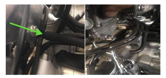
Left) There are 6 carb drain lines that attach to the carb bowls and come to a T. Remove the line at the T (right) Then remove the 6 carb drain lines from the carb bowls.
