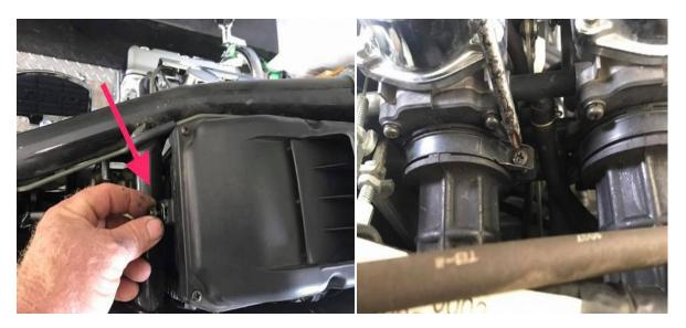
(left) Remove the bolt at the back of the airbox
