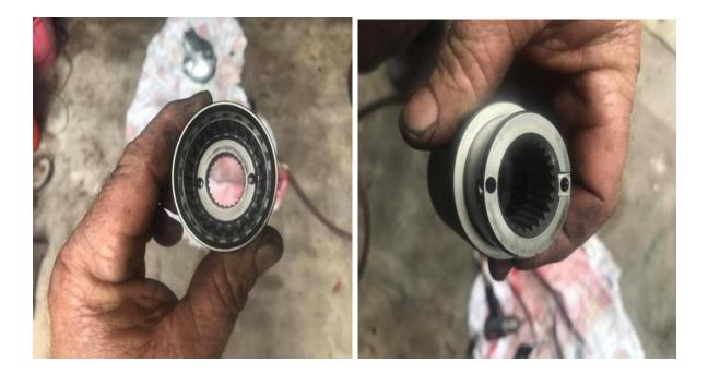
(left) Clean the cup up real good and be sure the holes are open and clean.
