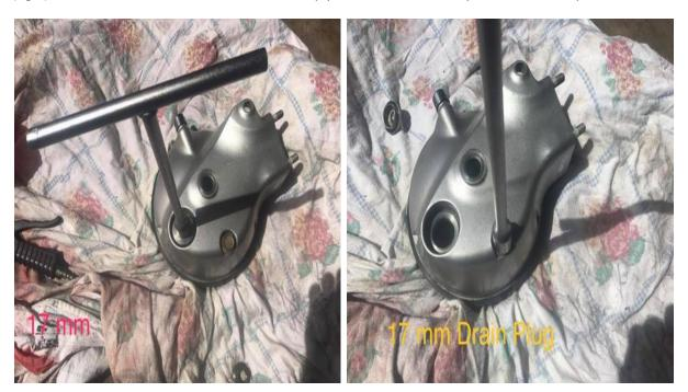
(left) Remove the fill plug with a 17mm socket
