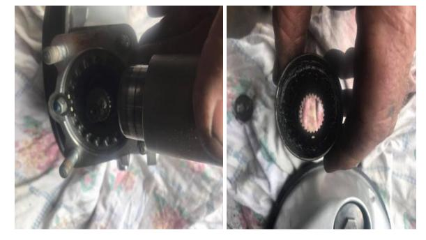
(left) Once the nut is removed you can pull the pinion cup off
