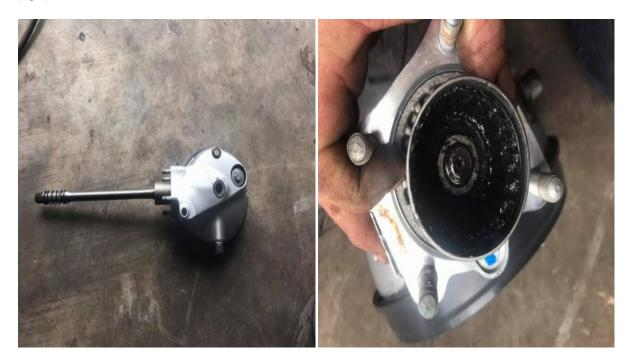
(left) After pulling the driveshaft out of the final drive I inspect the shaft and pinion cup splines.
