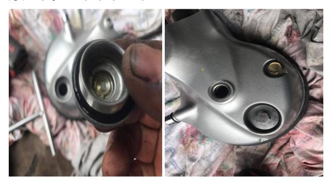
(left) I put a dab of oil on the o ring before I install it back on
