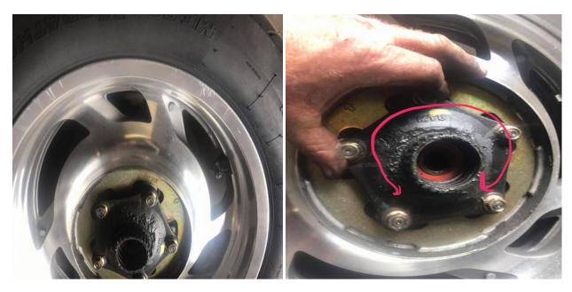
(left) Got the wheel off and notice quite a bit of grease leaking out around the splines. My first thought was the last guy didn't change the 3 o rings?(right) Trying to work it back and forth to see if there is any wear or movement in the wheel dampners. These are really tight.
