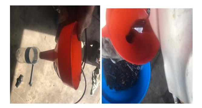
(left) I like to look at what comes out for metal particles and use a funnel into a water bottle (right) I pour the gear oil out of the final drive into the funnel to completely drain it.
