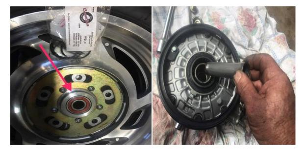
(left) Check the wheel bearings for smoothness and any movement and clean everything up (right) Pull the spacer out, one end is belled and the other is not. The small end goes in the hole  $1^{st}$ .
