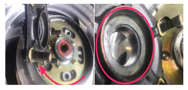
(Left) Pins where really dry which made it hard to get the drive flange off. The pins seat into the wheel dampers to cushion the jerk on and off the throttle. The dampers are about \$35 for new ones and very easy to change but these are really good.(right) The thrush washer is here and need to be sure it goes back on, if it shows wear replace it. I do mine every other tire change.
