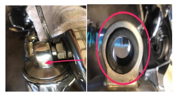
(left) Pry the top of the shock off the frame stud. It helps to take some of the weight off the wheel so it isn't under pressure and will come off easier.
