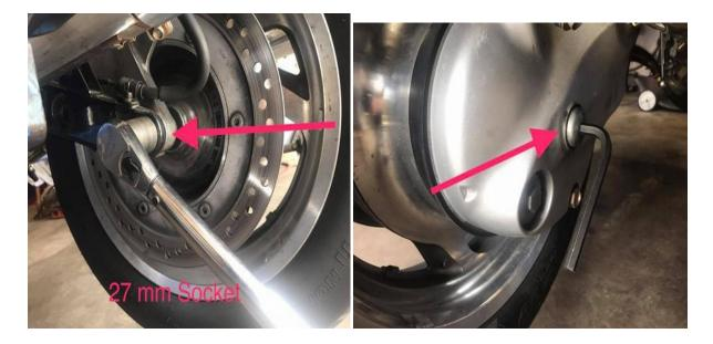
(left) Then I raise the bike so the tire is just barely setting on the floor and remove the axle nut.
