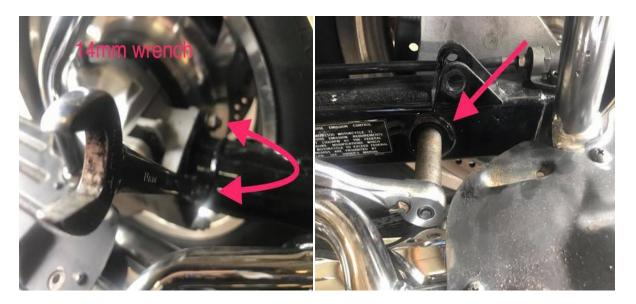
(left) Then I loosen the top driveshaft housing nuts. I don't remove them just loosen them so they still have a few threads left before coming off
