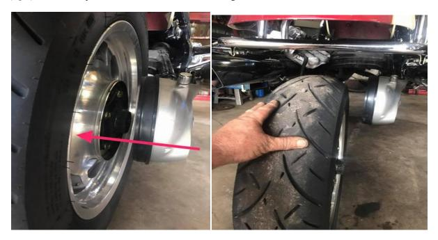
$\left( left\right)$  Pull the wheel to the left side until it comes out of the final drive splines
