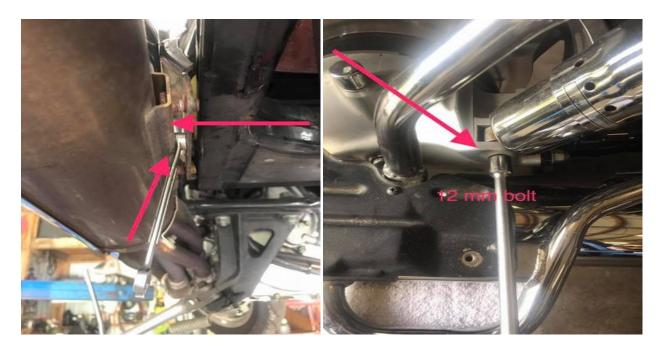
(left) I pry the mufflers out and stick a box end wrench in between the hanger and muffler to shim it out away from the swing arm slightly.
