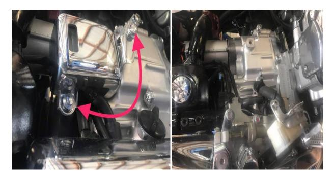
(left) Remove the rear brake master cylinder cover and mounting bolt.
