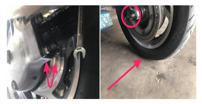
(left) I remove the bottom 2 nuts from the driveshaft housing but still leave the top as they were just loosened.
