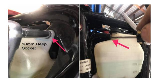
Next push the vent line off the top of the tank. Use caution not to break the nipple off the tank, it is plastic.
