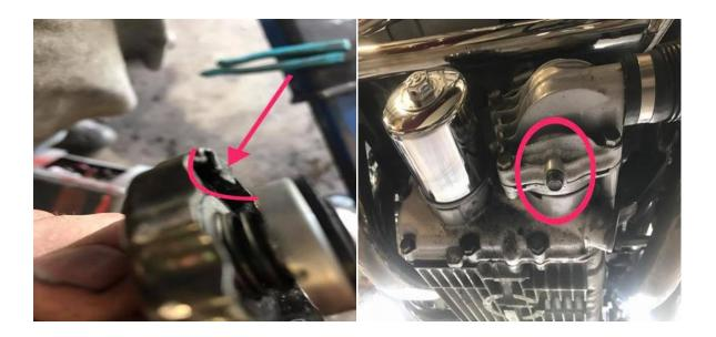
(left) I had to squeeze these tabs on both sides to make it seal better. Over time being taken, on and off the got to bent out some and just need a little bend back to get them sealing again. I like to round the outer edges slightly to make them easier to remove.
