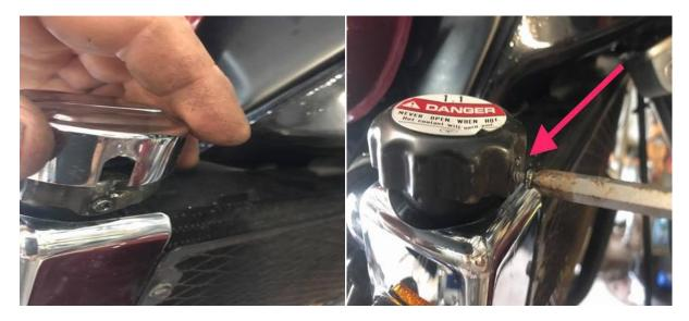
(left) Chrome cap is just held on by double sided tape so should pull off or pry a little up on it thru the opening by the Phillips head screw to get it started.
