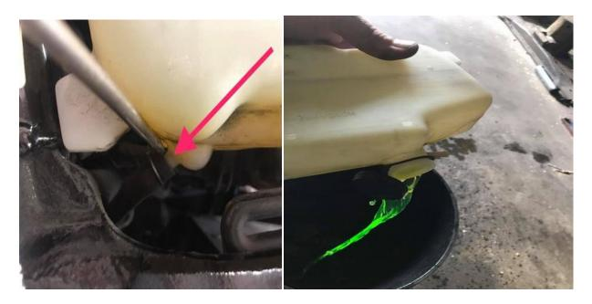
(left) I use a screwdriver and pry it off, it will usually come right off without even messing with the wire clamp. Be careful not to break off the plastic nipple on the tank trying to force it though.
