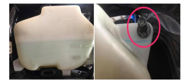
(left) Next we have to remove the reservoir bottle behind the Left side cover under the seat to drain and clean it.
