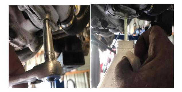
(left) Have something for the old anti freeze to drain in when you remove the bolt. About 3/4 of a gallon will be comin to ya. You have to leave the top radiator cap off or you'll be waiting hours for it to drain.
