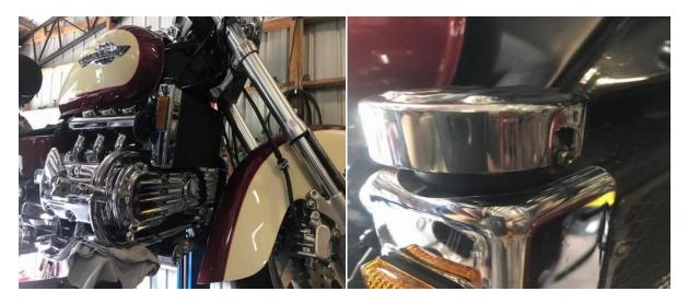
(left) Remove the radiator cap from front right side of bike
