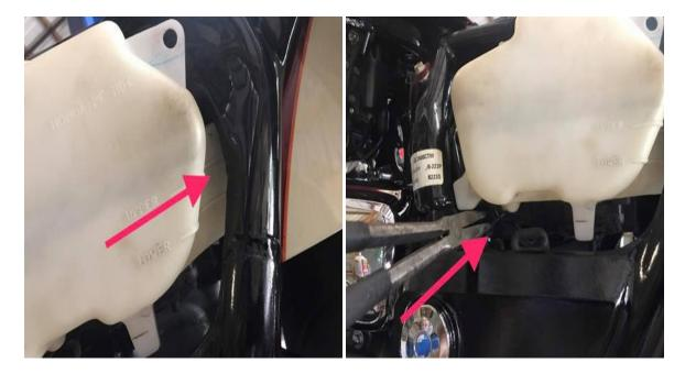
(left) Slide the reservoir tank back into place. The tab needs to slide in behind the frame
