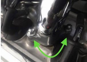
(left) 1st thing I do is to remove the chrome covers off the choke slides. Not worth scratching and it makes it so much easier to remove the intake runner bolts. By removing these it allows you to be able to use a long extension down to the bolts to remove them very easily. Worth the 3 little screws it takes to remove them
