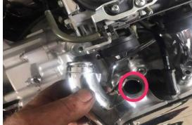
(left) Once all the clamps are loose and all 6 bolts from the bottom are removed, grab the first one at the bottom and lift the carbs while pulling out and up on the intake runner. It will pop right out. Some may have a vacuum line attached to the back of them to remove also
