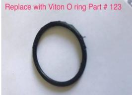
(left) Turn it over and you'll see the o ring that needs to be removed and replaced. Clean the surface real good before putting the new o ring on. Just above the red arrow you see a little nipple sticking out, make sure the passage is clean inside these also. Depending if your bike has been desmogged or not you may have some lines still to connect to them. But even if they are capped it's a good idea to clean them so if you decide to sync the carbs it will be clean.
