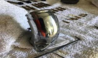
(left) Once all are removed and the holes are plugged I clean the mating surface real good for a tight fit. I smear a little Vaseline around the holes to help the runners slide back in when I replace them
