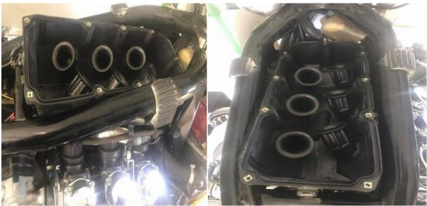
(left) I keep pushing and working the horns around anything they get hung on till I get it all down in the hole. (right the snorkel tubes are what I was talking about. I twist the snorkel tubes so as to make sure none of the horns are folded under and won't make a good seal.
