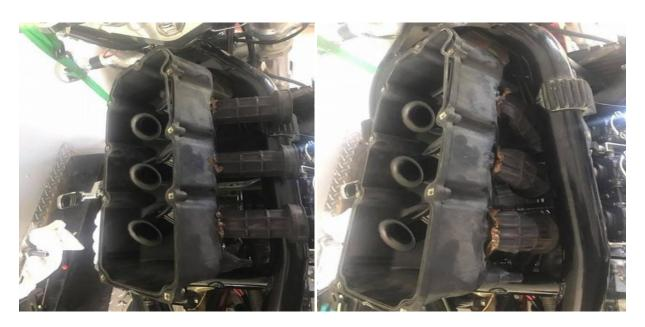
Left) I lay it in with one side of the tubes in the hole (right) Then I push the other horns down in.
