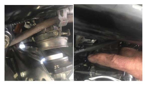
(left) I loosen the claps all the way up and slide them on and up out of the way. I leave them off when I'm pushing it in the hole and then look at them As I put them on to see the best way to position them for tightening when I install them on the horns
