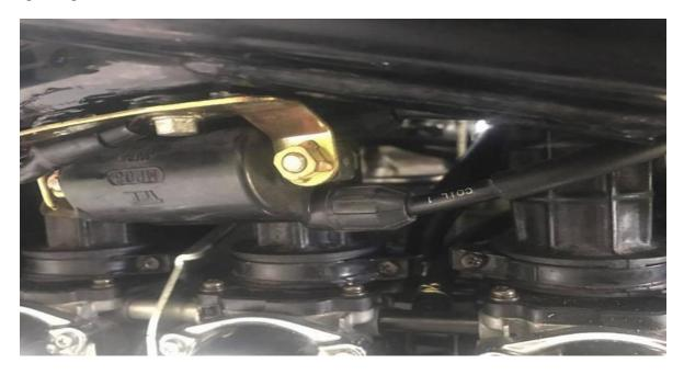
Make sure the clamps go on easy and straight and the horns are all the way down and tighten the clamps
