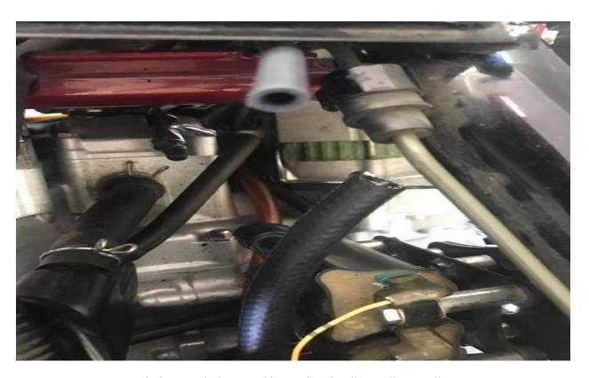
Connect the hoses to the bottom with some long handles needle nose pliers.
