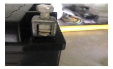
I fold the strip and cut it off so it gives a little shim under those floating nuts that come in the battery. What the shim does is raise the nut up so that the screw will start into the nut. Without the shim the screw is just shy of being able to reach the nut once you put the cables on top of the terminals. Don't believe me? Leave it out and get back with me once you get done cussing that nut out for not holding still.
