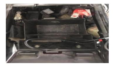
This is with the old battery removed and getting ready to receive a brand new battery
