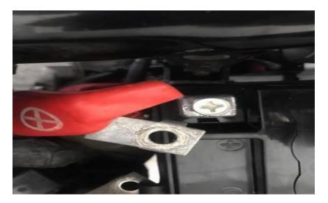
The (+) side is for the red terminal or the wire that goes to the starter solenoid.
