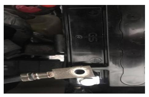
You'll see the (-) for negative or ground and that's where the black wire or the one that goes to the back of the engine for a ground goes. Clean the terminals off good so they make a good connection.
