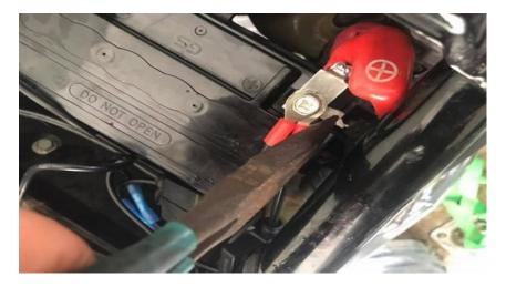
Once you get the screws started you can remove the paper shims you put under the nuts
