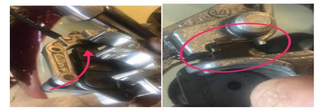
(left) Put the first pad in with the metal against the pistons, pad Part facing out and the hole where the pin came out.
