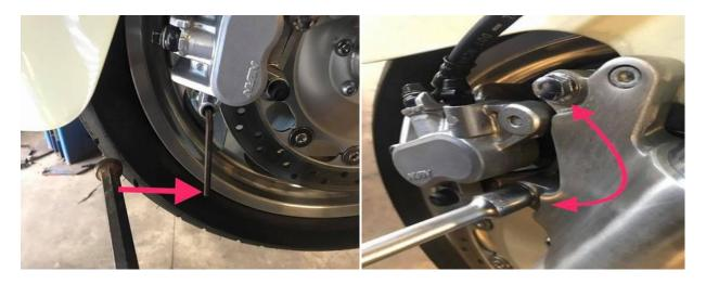
(left) Hold in tightly on the Allen wrench and give the wrench a wack to break it free. I don't remove it yet just make sure it's broke loose. Easy to have the bikes hold it while you are trying to loosen it then trying to hold it and twist it.(right) Next remove these 2-12mm bolts and hold the caliper from falling when you remove them.
