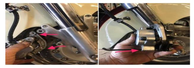
(left) Pull the caliper out from behind the mounts.
