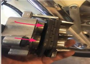
(left) Remove the rubber boot and pad clip
