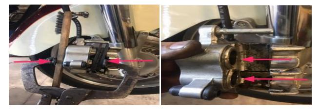
(left) If your using 2 clamps you can just tighten them down evenly as it squeezes back together but I'm using only one so have to alternate back and forth between the 2 pistons.
