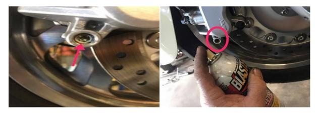
(left) After the cover screw is removed you'll find an Allen head you need to clean the head out real good so your Allen wrench will fit all the way into the head nice and tight.
