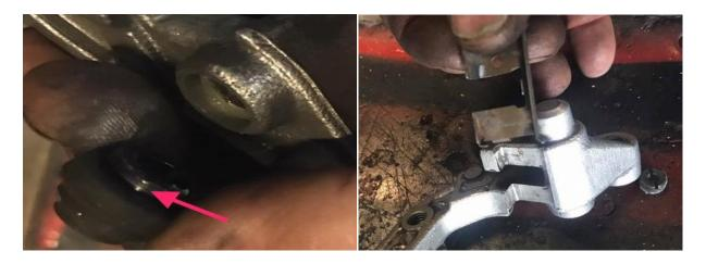
(left) Put a dab of silicone grease or dielectric grease on the end of the rubber plug so it will seal the dirt and moisture out. (right) Put the clip back in.
