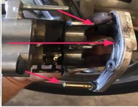
(left) Separate the 2 pieces of the caliper
