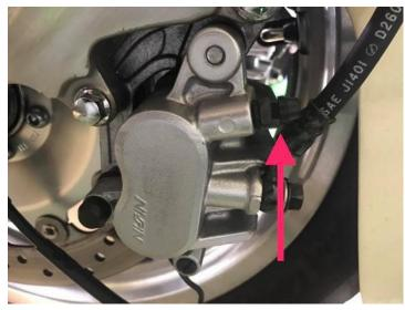
Locate the bleeder nipples on the calipers. I always start with the farthest one which would be the left side then do the right. 2 calipers on the front brakes
