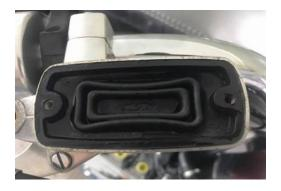
Under the plastic cover is a rubber diaphragm that as the fluid gets low it expands and follows the level down to keep air out.
