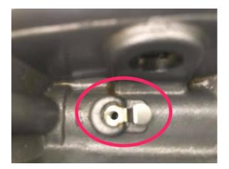
Once all the fluid is out need to clean the cylinder out. Don't lose this little piece and note how it is installed
