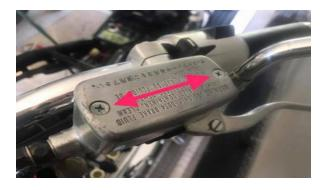
Starting with the front brakes the master cylinder is on the right side of the handlebars. Cover all areas around it with rags to keep any brake fluid from spilling on your motorcycle, it will ruin your paint
