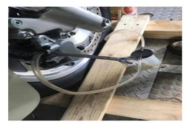
I have an old brake bleeder cup but any container will work if you put a little brake fluid in the bottom and keep the other end of the hose down in it so it can't suck air.
