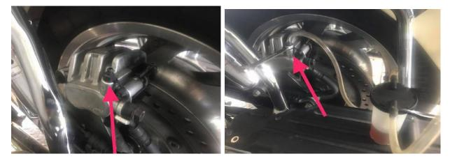
Locate the bleeder nipple on the back left side of the wheel Add the 10 mm wrench and tubing to the nipple
