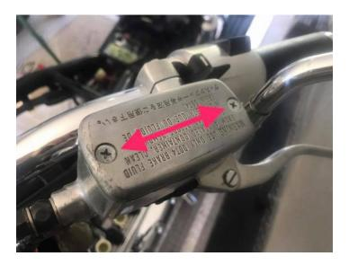
Remove the cover off the clutch master cylinder on the left side of the handlebars
