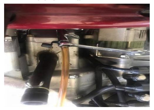
Attach a 10 mm box end wrench and a piece of clear tubing run down to a container or brake bleeding canister
