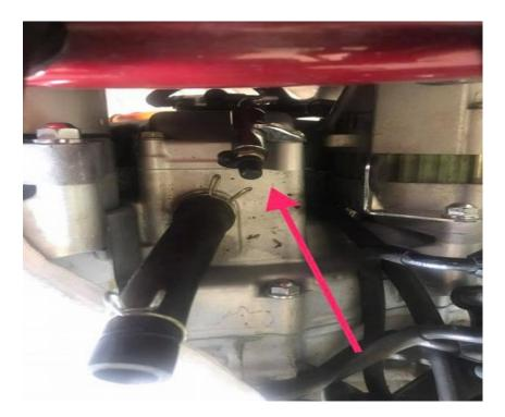
Locate the clutch bleeder nipple
