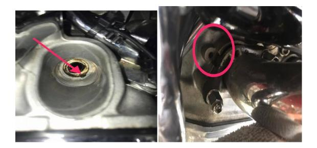
(left) Here's a picture of the hole after the plug has been removed.
