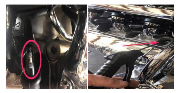
(left) Each plug wire is marked as to what cylinder it goes to. On the left side of the bike you have starting from the front of the bike going toward the rear 2,4,and 6 cylinders. On the right side you have 1,3 and 5.
