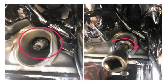
(Left) Put the plug back in the hole and get it started so it's not Cross threaded.
