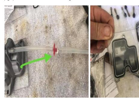
(left) Also has a neat little test tube and plate to check for leaks. Got to make sure this little red diaphragm is going the right way or you won't get any suction out of it.
