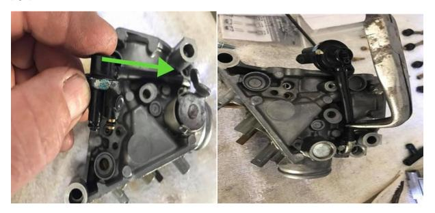
(left) I stuck a little Vaseline on the metal vacuum tube so the rubber line would slide on.
