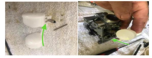
(left) Clip the needle valve into the float tab
