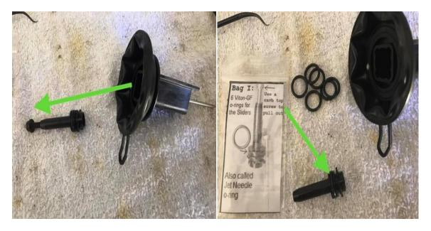
(left) It should pull right out, no need to remove the needle just replacing the o ring  $\frac{1}{2}$
