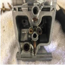
(left) Install the slow jets and snug down with screwdriver (right) Don't over tighten or you'll break the top.
