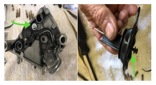
(left) Position the cut valves into place and install the screw
