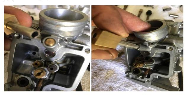
(left) Using the special tool or screwdriver if you cut slots, screw it all the way in till it just touches bottom
