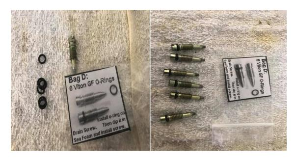
(left) 1st bag I started with was the carb drain screws. Replaced the o rings around the head (right) Pretty simple job, I use a little Vaseline to help them slide.
