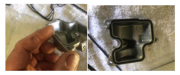
(left) After testing I added a little Vaseline to the groove for the gasket to set in and hold in place (right) Press the gasket into the groove making sure it is on all the way around.
