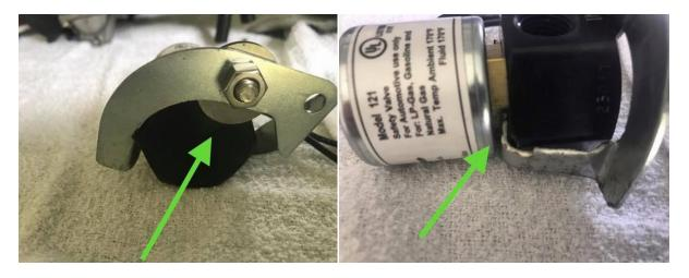
(left) I used a large flat washer on the bottom to hold it from falling down
