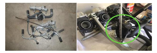
(left) When we do a desmog on the Valkyrie this is all the clutter we remove. It nothing but extra weight, engine clutter and future vacuum leaks to maintain. By removing it we lose or gain nothing extra in performance just a clean up of unnecessary parts to eliminate future maintenance.
