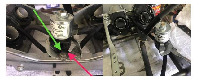
(left) And used the head of a bolt that secures it to the carb frame to keep it from sliding out. The red arrow shows the washer on the bottom holding it from falling down
