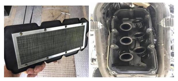
(left) This is the bottom side of the filter that goes down toward the engine when you replace it
