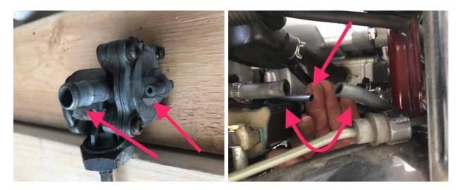
(left)This is the OEM style petcock, the large fitting on the left goes to the fuel supply line and the smaller fitting on the right goes to the vacuum line come off the #6 cylinder intake runner.
