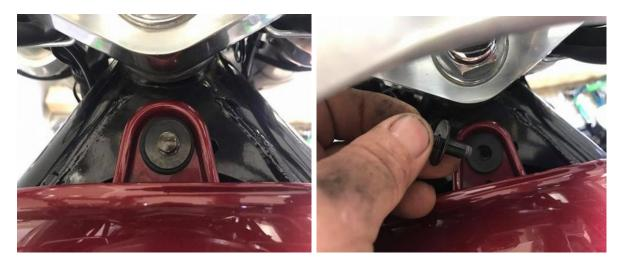
(left) Then remove the 8mm bolt at the front of the tank
